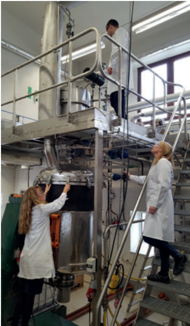
Figure 1. RISE Processum steam explosion device. From left to right: Julia Forsberg, Roger Molinder and Karin Johnson. The equipment upside is a 40 L reactor above a 1000 L explosion vessel.
